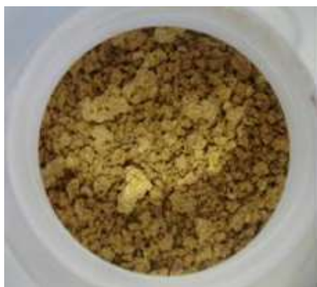
Fig. 4. Calcine obtained with the appropriate adjustment and operating parameters
